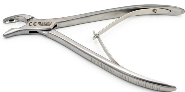
Trotter Bone Rongeur Angled 10mm Bite with Compound Action
